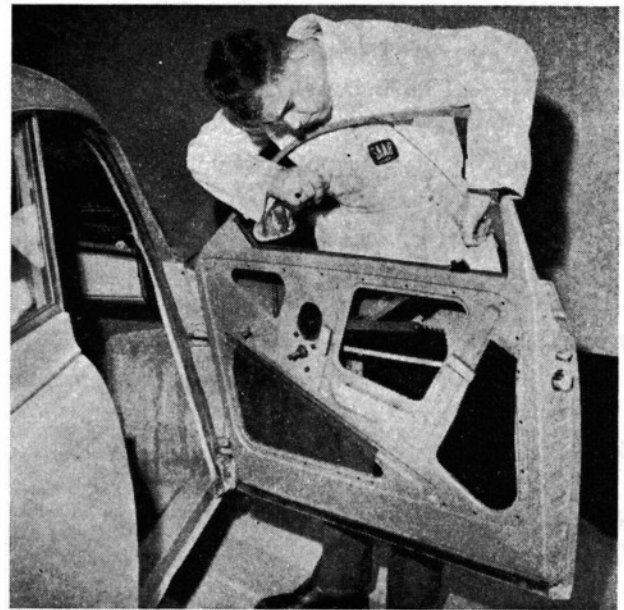
Removal and installation of door glass
