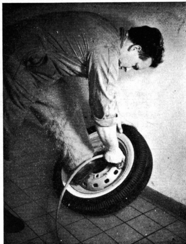
Pressing in tire bead
