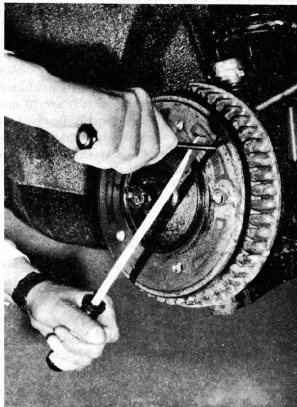
Readjusting brake shoes, type III
