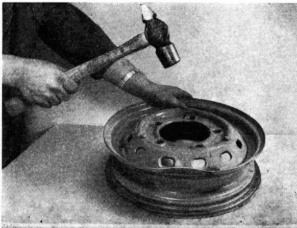
Straightening wheel rim
