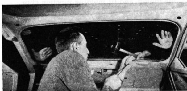
Fitting windshield strip with leather thong
