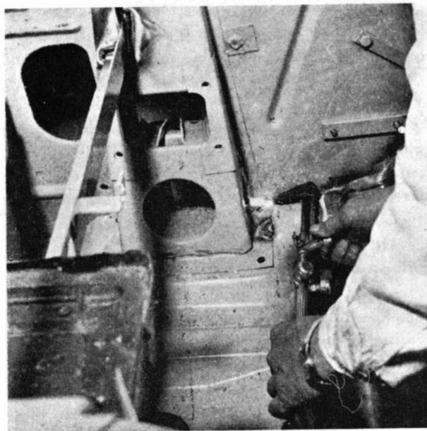
Cutting away wheelhouse and suspension-arm bracket
