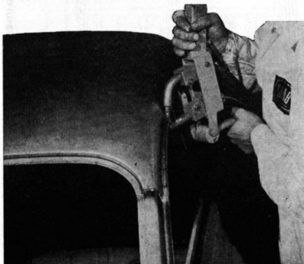
Fitting and welding of roof sheet
