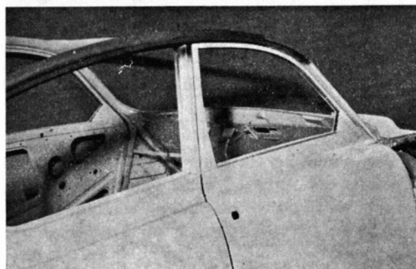
Fitting new roof rail and molding
