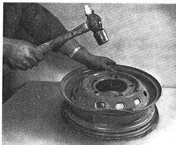
Fig. 8. Straightening rim flange
