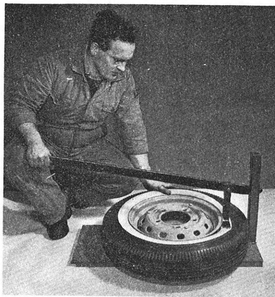
Fig. 9. Freeing bead from rim flange
