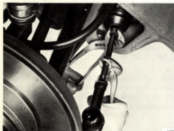
Adjusting the tie rod
