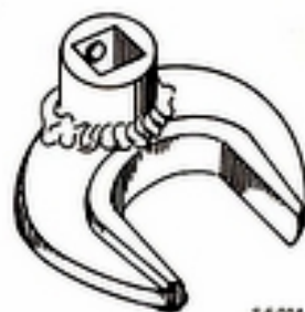
89 96 480 Wrench, removal and installation of ball joint, servo assisted steering
