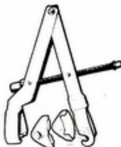
89 95 839 (A1) Spring tool cpl., removal and installation of front spring
