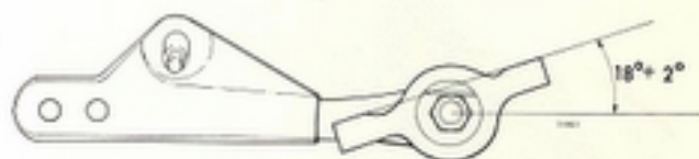
Angle between lower control arm and bearing
