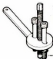
89 96 258 (A0-2) Steering wheel puller
